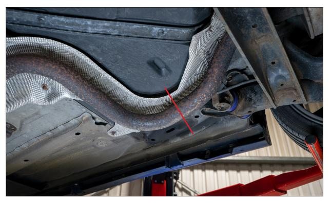
The original exhaust system requires cutting to remove. We recommend cutting it in the centre of the small straight section in front of the rear axle.
